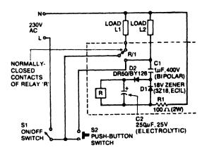
When AC mains power is switched on through S1, power is applied to load L1 via the normally-closed contacts R/1 of relay R. If S2 is pressed momentarily, power is instantly applied to the load L2 and simultaneously to the electronic circuit.
